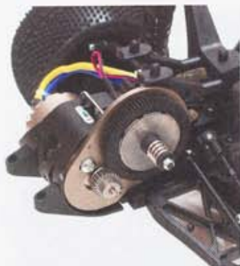
Left: The brushless ready twin plate slipper allows the user to help protect the driveline, and adjust how power is fed to the rear wheels
