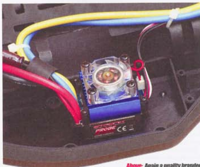
Above: Again a quality branded Etronix Probe ESC capable of running a 12T motor and LiPo safe to boot!
